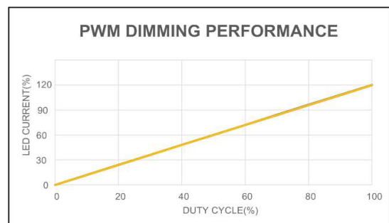
Figure 10. Current accuracy vs PWM dimming
